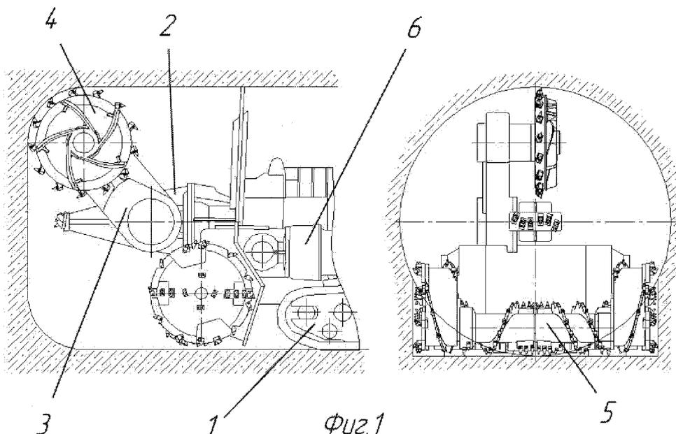
(57) Abstract: The invention relates to mining machines. A mining machine comprises a chassis (1), a working member (2) having an arm (3) and a cutting device (4), and a lower breaking and loading device (5) with a drive (6). Technical result: coordinated operation of a working member and a lower breaking and loading device having an optimal conveyor design during the excavation process.
